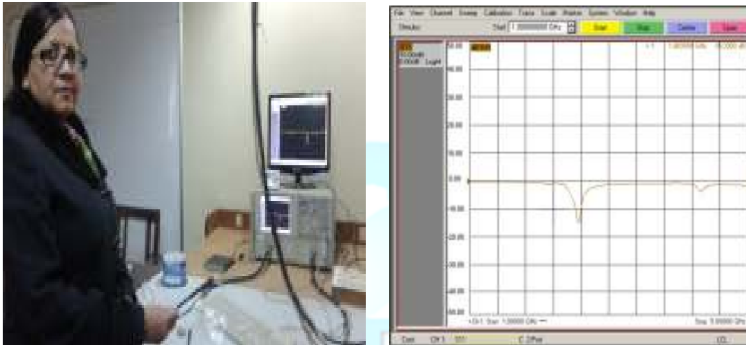
Figure13. Proposed antenna while measuring result on vector network analyzer in IIT Kanpur Lab
